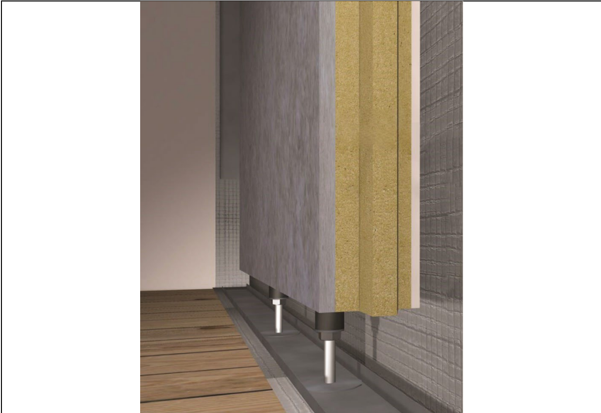
Figure 3 The Matilda's Blanket Internal Wall Insulation System – dampers
